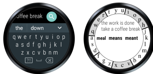
Figure 4.2: When entering the phrase “the work is done take a coffee break” with a smartwatch QWERTY, only the last 10 characters are visible (left), while the whole phrase is visible (37 characters) with SwipeRing (right). Besides, there is extra space available below the floating suggestion bar to display additional information.
