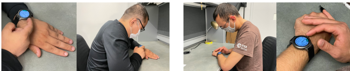
Figure 3.4: Participants entering text with the manual (left) and the automated crown-based keyboard (right) in the second user study.
