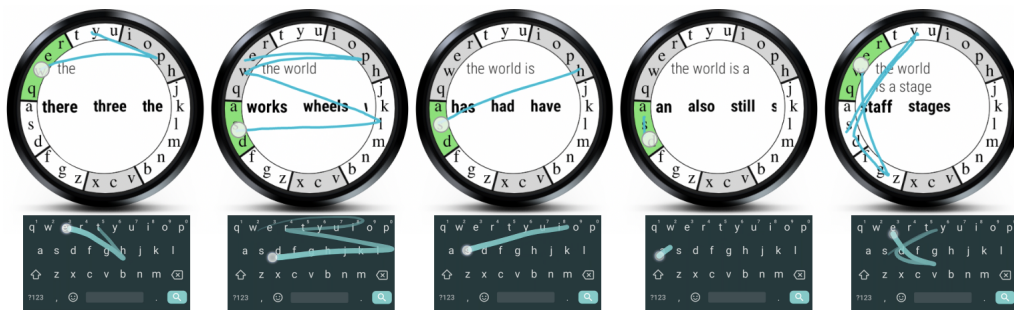
Figure 4.1: SwipeRing arranges the standard QWERTY layout around the edge of a smartwatch in seven zones. To enter a word, the user connects the zones containing the target letters by drawing gestures on the screen, like gesture typing on a virtual QWERTY. A statistical decoder interprets the input and enters the most probable word. A suggestion bar appears to display other possible words. The user could stroke right or left on the suggestion bar to see additional suggestions. Tapping on a suggestion replaces the last entered word. One-letter and out-of-vocabulary words are entered by repeated strokes from/to the zones containing the target letters, in which case the keyboard first enters the two one-letter words in the English language (see the second last image from the left), then the other letters in the sequence in which they appear in the zones (like multi-tap). Users could also repeatedly tap (instead of stroke) on the zones to enter the letters. The keyboard highlights the zones when the finger enters them and traces all finger movements. This figure illustrates the process of entering the phrase “ the world is a stage ” on the SwipeRing keyboard (upper sequence) and on a smartphone keyboard (bottom sequence). We can clearly see the resemblance of the gestures.
