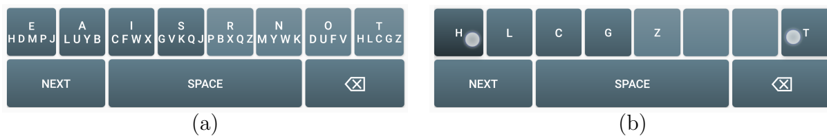
Figure 5.3: The Senorita chorded keyboard used in the experiment. It enables users to enter text by pressing two keys simultaneously using the thumbs. (b) Pressing a key highlights all available chords for the key.
